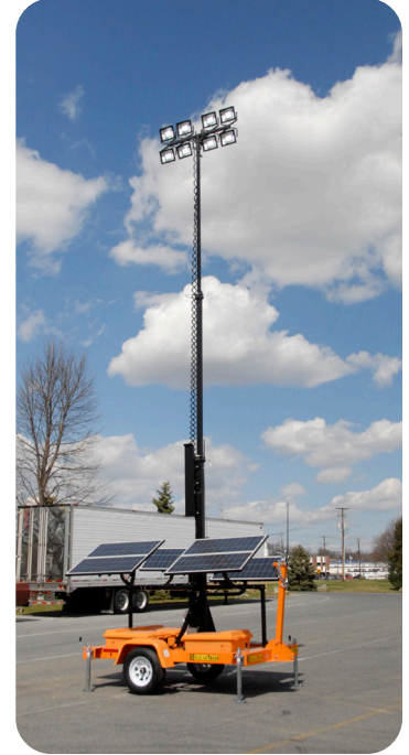
30' Light Tower with 4 or 8 50-watt LED Lamps
